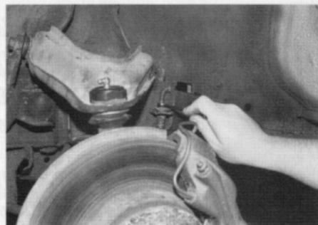
*Connect the rubber hose to the steel brake line at the framerrail. Be sure to reinstall the clip securing the end of the hose to the tab on the framerrail.*
