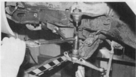
*Install and torque the replacement lower-ball-joint nut and cotter pin.*
