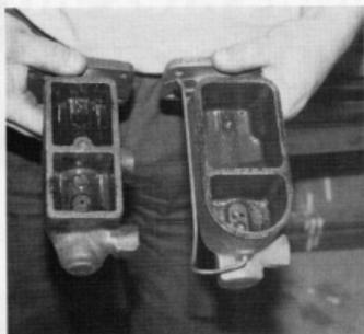
The difference in reservoir configuration between the drum-brake master cylinder (left) and the disc-brake master cylinder is obvious. The larger reservoir on the disc-brake master cylinder feeds the front brakes. Though it's not apparent in this photo, the reservoirs in the disc-brake master cylinder are deeper than those in the drum-brake master cylinder.
