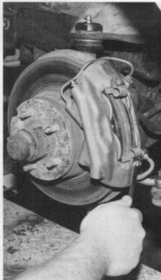
*The clips are made of spring steel. They serve to retain the pads in the caliper and keep the pads from rattling.*
