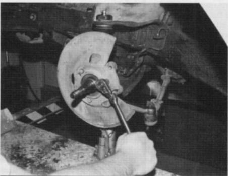
*Install the disc-brake dust shield next.*
