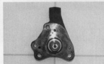
The line between the centers of the lower-ball-joint attaching holes is perpendicular to the vertical centerline of the knuckle. Therefore, it's possible to move the knuckles from side to side with no effect on steering geometry or the operating angles of the ball joints.
