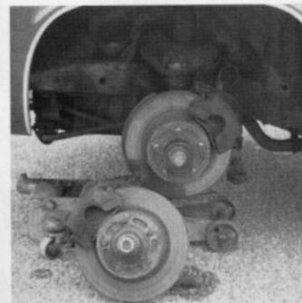
This '71 A-Body has been fitted with '73-and-up single-piston disc brakes. From the factory, orientation of the caliper on '73-and-up A-Bodies was toward the front of the rotor (as shown by the assembly on the ground). This creates a small problem on some applications. If your '72 or older car has a sway bar, the sway bar links want to occupy the same space as the calipers. The solution is to swap knuckles, calipers, and caliper mounting brackets from side to side.
