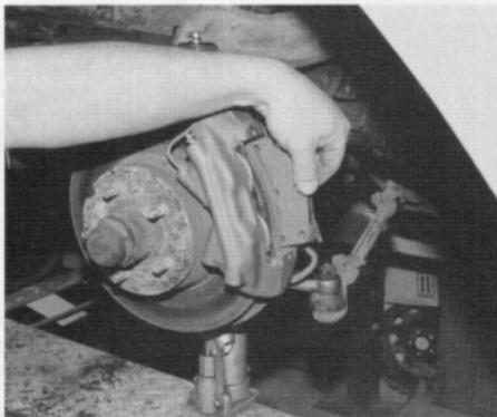
*With the caliper pistons at the bottom of their bores, the new disc-brake pads are dropped into place.*
